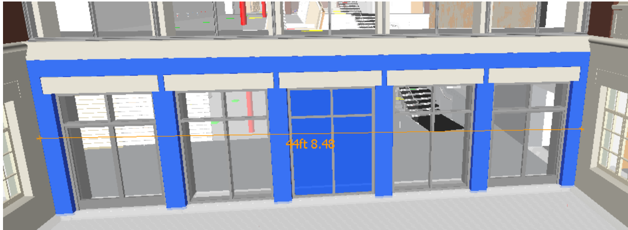
Figure 31 Atrium South Curtain Wall with a Width of 45 feet
