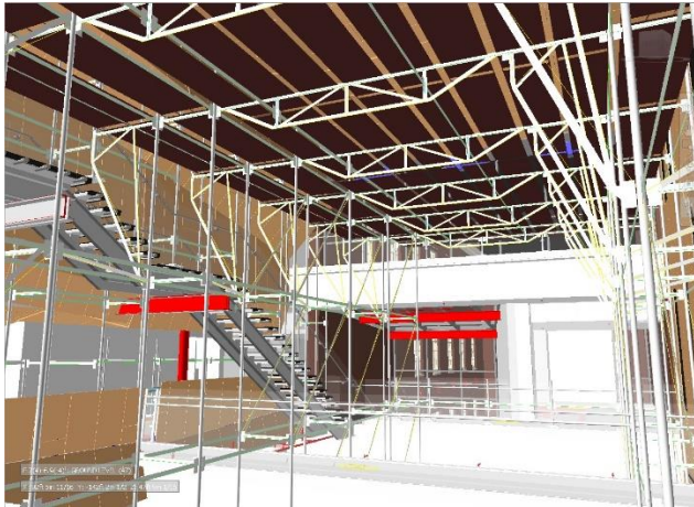
Figure 27 Atrium Space Depicting Congestion of Scaffolding, Stair Installation, and Architectural Screen Wall
