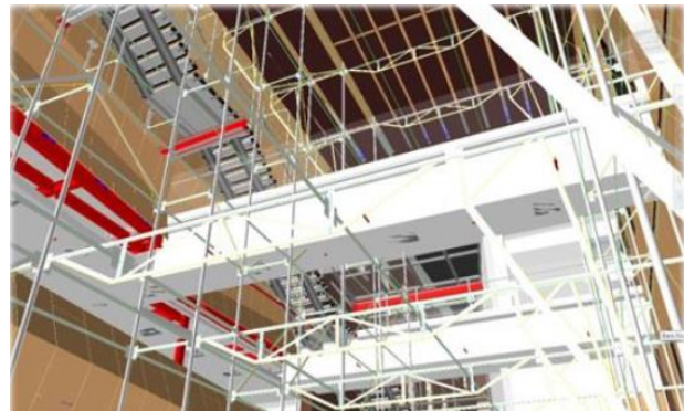
Figure 9 Atrium Space Showing Congestion of Scaffolding, Stair C, and Screen Wall Installation
